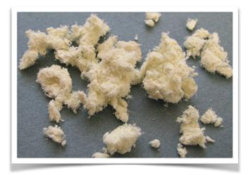
Kevlar® stop-leak (fibrillated 2 mm Kevlar® fibers)
