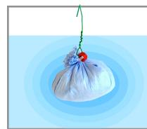
Treatment chemicals (in powder form) are placed on the diffusion membrane. Edges are gathered and sealed tightly with a zip-tie. Suspended in a system reservoir, water slowly diffuses across the membrane, dissolves chemicals and the resulting treatment solution slowly diffuses across the membrane into the reservoir.
