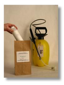
A converted garden sprayer suffices. It connects to any valve on the system having garden hose thread.
